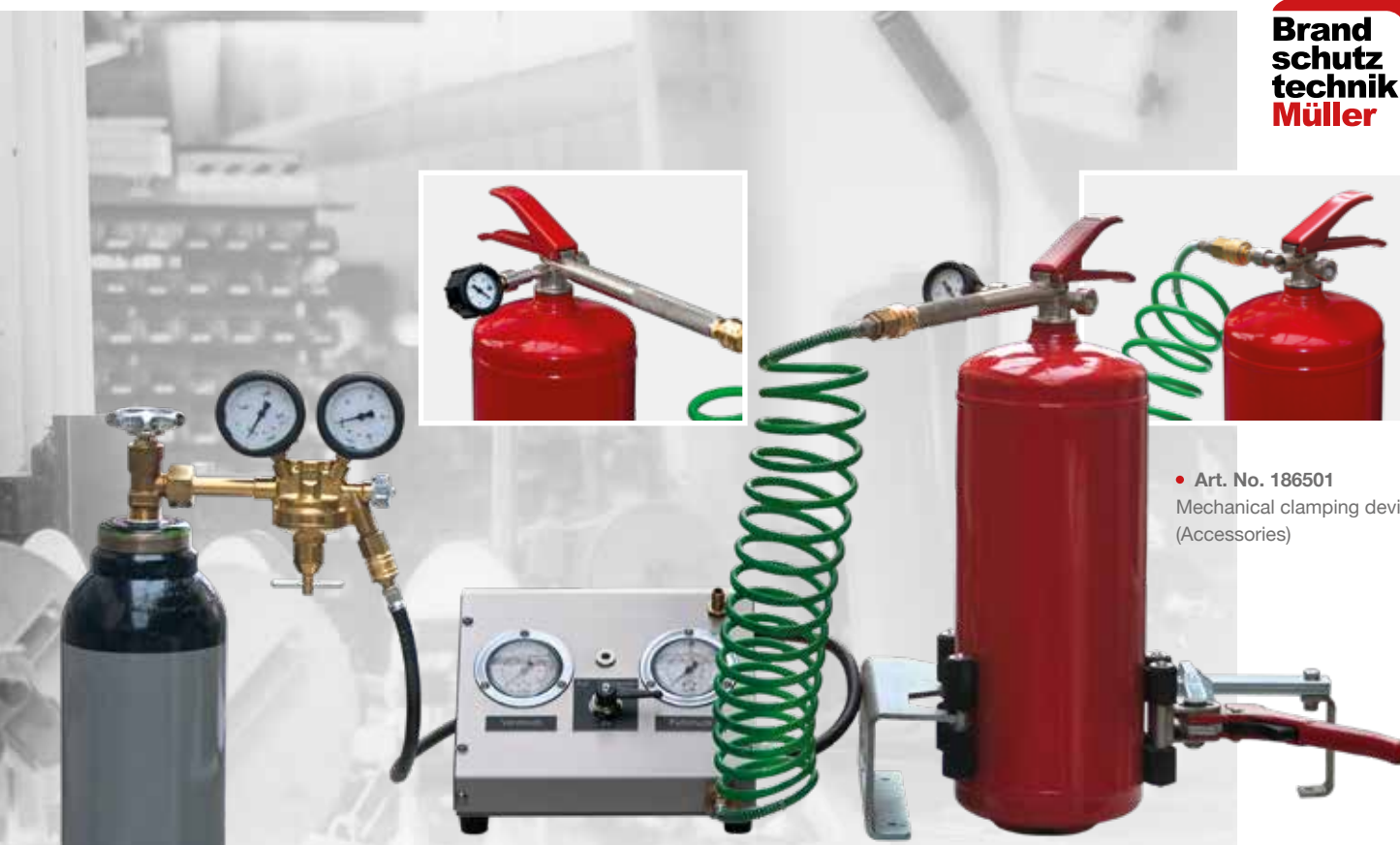
• Filling of a stored pressure fire extinguisher from the nitrogen storage bottle.
