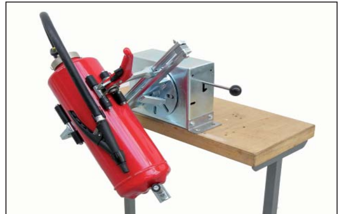
Fig. 2: The DSV stationary clamping device is fixed to a work bench. The clamped fire extinguisher can be turned 360° and locked in steps. Thus, all work can be carried out safely and effortlessly in no time at all. The height adjustment ensures an optimal momentum balance when turning the fire extinguisher.
