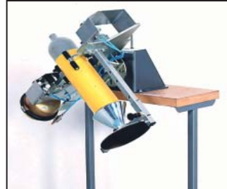
Fig. 11: The SVPA ROTATABLE clamping device works like the SPVA described opposite except that it can also be turned 360°. The clamping device can be locked every 45° in steps. Thus, all work
