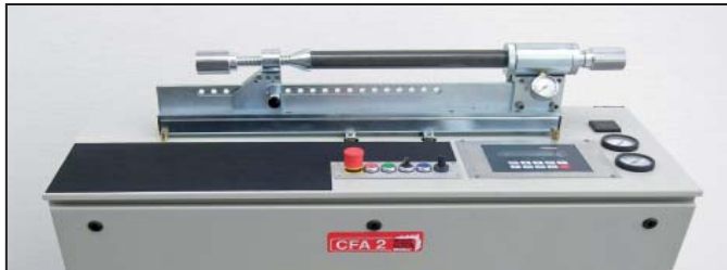
Fig. 3: The F1M universal filling head for internal CO 2 cartridges with universal attachment flange and the CO 2 connection hose for supplying the unit are supplied as standard items.
