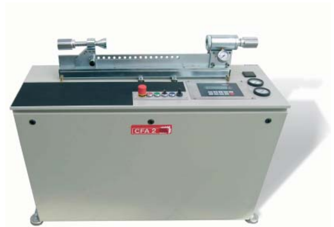
Fig. 1: The CFA 2 is a carbon dioxide filling unit with adjustable filling output and a speed-controlled motor. The F1M universal filling head is mounted on an electronic weighing cell. The control panel is ergonomically located for comfort and convenience.
