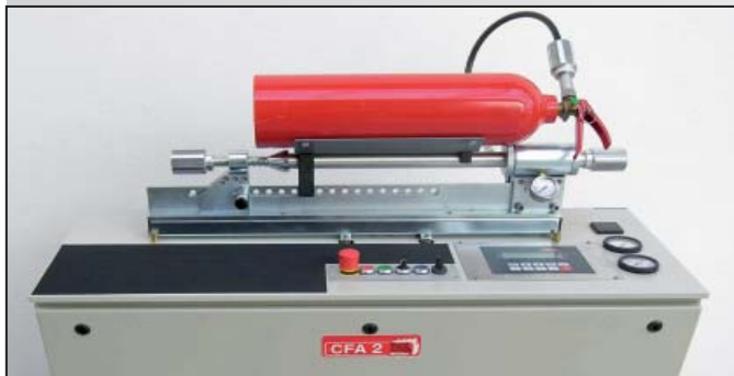
Fig. 5: F3 filling head for 2 to 6 kg CO 2 fire extinguishers Art. No. 186104
